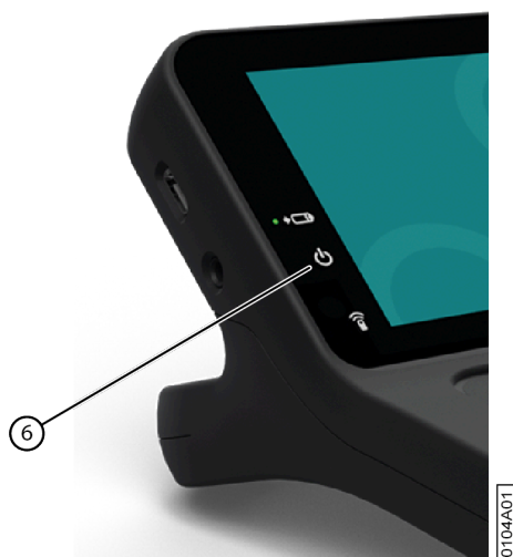
Figure 7: Viewing the power status
