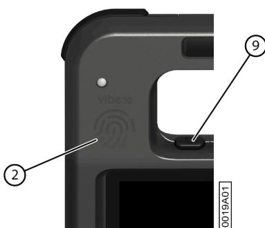
Figure 12: On/off button and wake-up sensor
