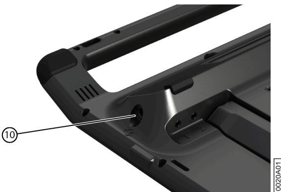
Figure 5: Connection for charging the device
